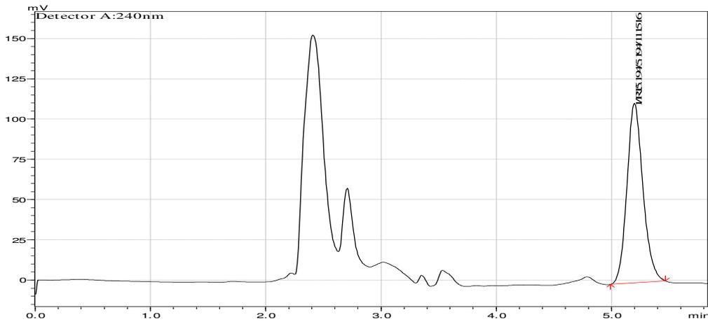
Figure: 3 Chromatogram of sodium cromoglycate and plasma
