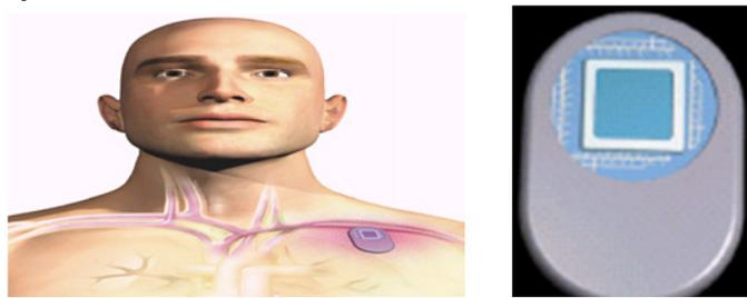
In this device contain a silicon microchip that was a 1.7 cm square with a height of 0.31 mm and contained 34 reservoirs. The drug releasing chip could potentially contain up to 1000 drug reservoirs, each covered with a thin gold film.
