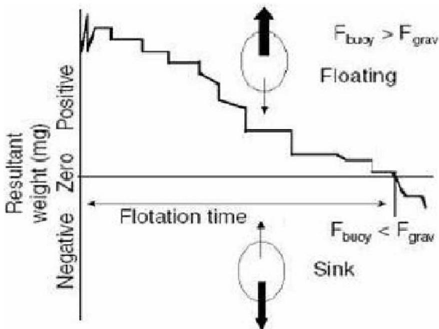
$$F = F_{\text{buoy}} - F_{\text{grav}} = D_f g V - D_s g V \quad F = (D_f - D_s) g V$$
