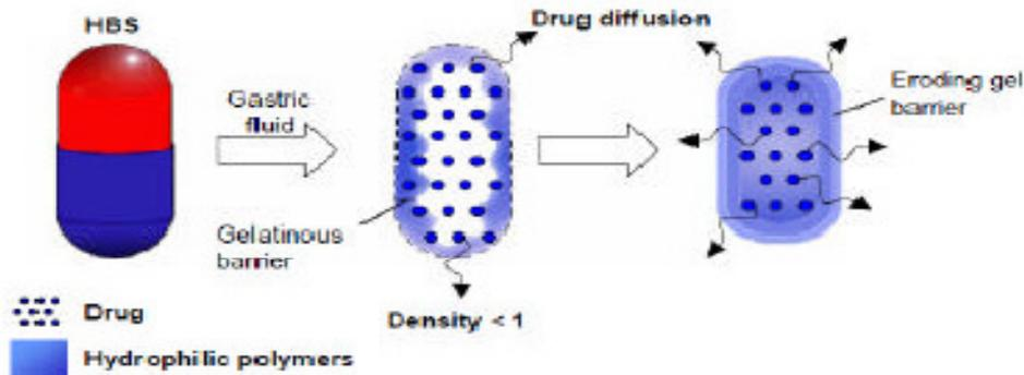
**Drug is released by diffusion and erosion of the gel barrier.**
