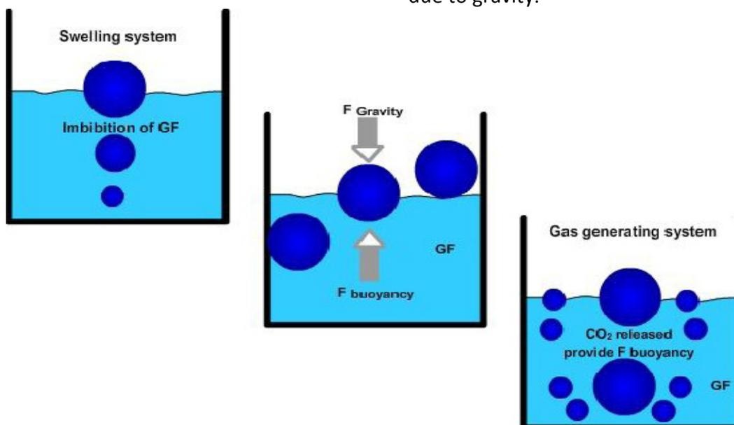
**Figure 6:** Mechanism of floating drug delivery system
