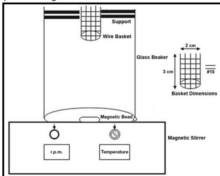
Figure.3- Modified disintegrating apparatus
