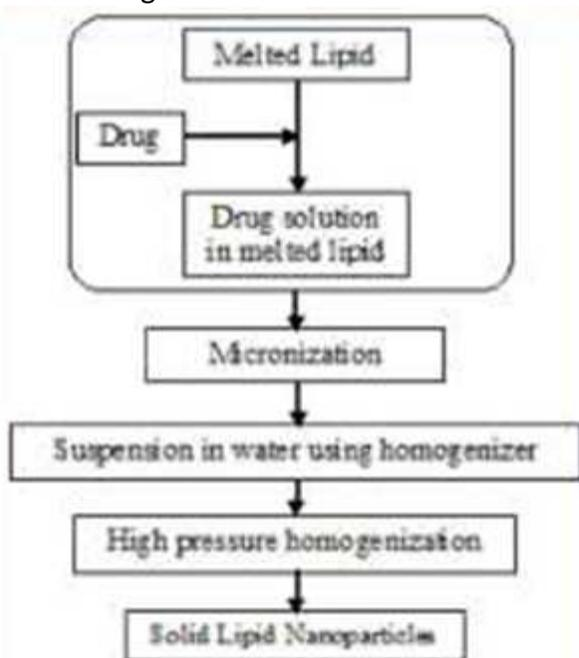
**Fig 4:- solid lipid nanoparticles by cold homogenization**
