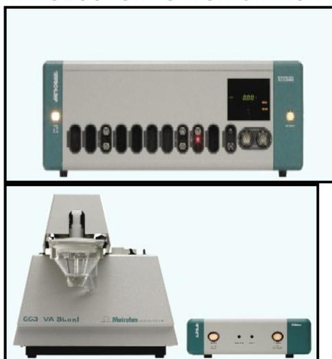
Electrochemical workstation- PG STAT 30 with 663 VA Electrode stand (Metrohm)
