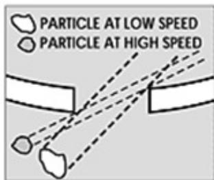
Figure 2.6.: Influence of the rotor speed to particle size<sup>19</sup>
