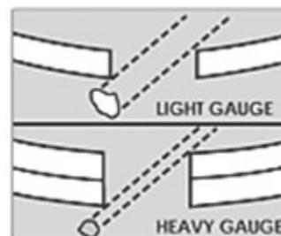
Figure 2.7.: Influence of the screen thickness to particle size<sup>19</sup>
