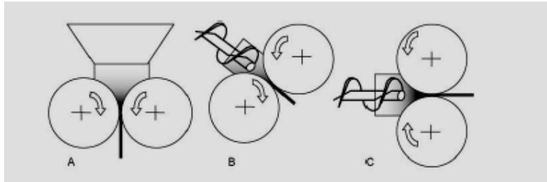
Figure 2.3.: Configuration of roll compactor
