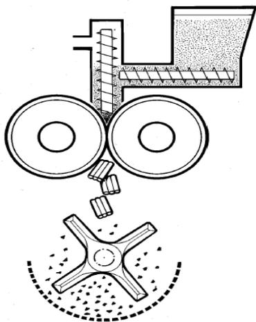
Figure 2.1.: A typical roll compaction process
