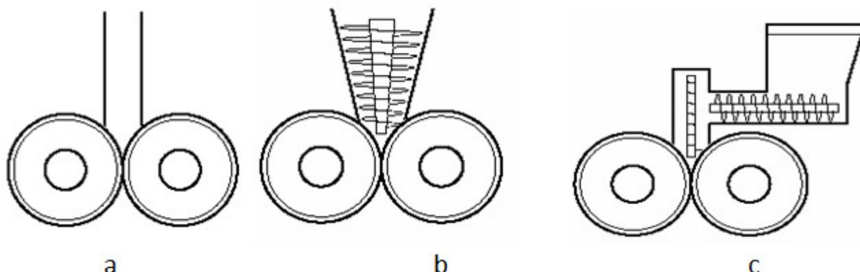
Figure 2.5.: Different feeding system: a) gravity feeder, b) single screw feeder, c) double screw feeder<sup>16</sup>
