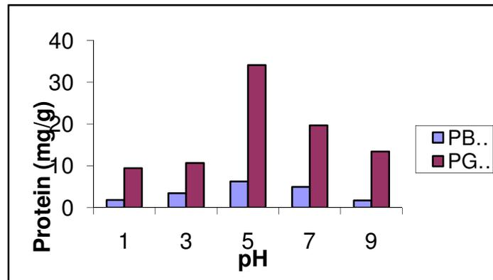
**Fig 2 Effect of variation of initial pH of SSF medium on the protein yield by *A. niger* Temperature**
