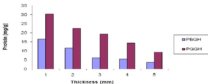
**Fig 4 Effect of thickness on the protein yield using *A.niger* by SSF**
