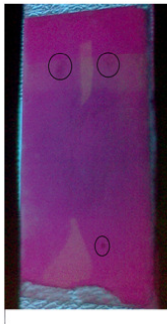
Fig 4: TLC plate of petroleum ether extract at 254 nm UV light
