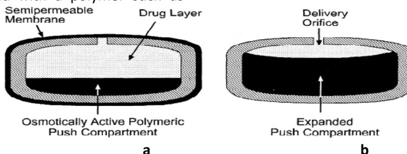
**Fig. no. 5 Schematic of OROS "Push-Pull" System (a) Represents the pump before operation. (b) Represents the pump during operation.**
