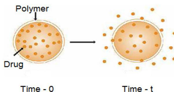
**Fig. no. 2 Schematic representation of diffusion sustained drug release**
