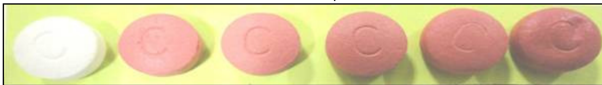
(C) Uncoated tablet (extreme left) with 4 % Kollicoat® Protect coated tablets after 0, 1, 2, 3 & 7 days
