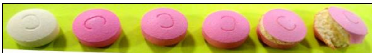
(B) Uncoated tablet (extreme left) with 4 % Aquarius® MG coated tablets after 0, 1, 2, 3 & 7 days
