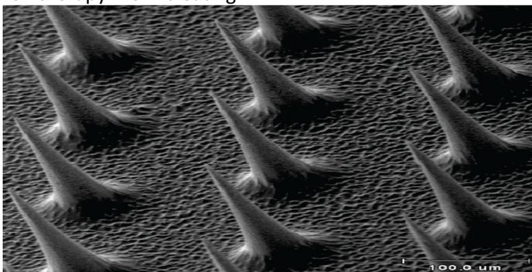
**Fig.2** Solid silicon microneedles
