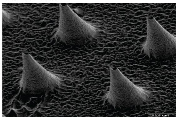
**Fig.3** Hollow metal microneedles [29]
