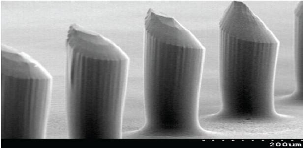
**Fig.4** Biodegradable polymer microneedles<sup>[29]</sup>
