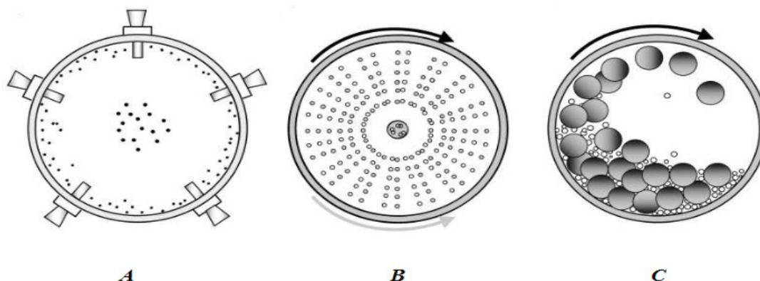
**Fig. 2 Cross-sections of 3 mills commonly used to create micron-size particles.**
