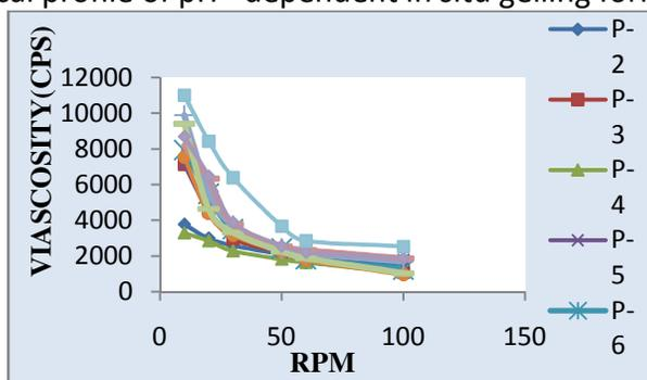
**Figure 6:** Rheological profile of pH - dependent in situ gelling formulations (Gels)
