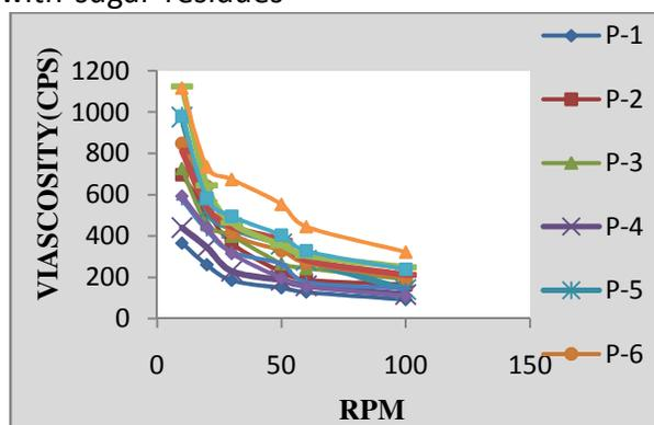
**Figure 5:** Rheological profile of pH - dependent in situ gelling formulations (Solution)
