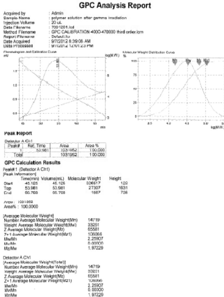
Figure 5: GPC after gamma irradiation
