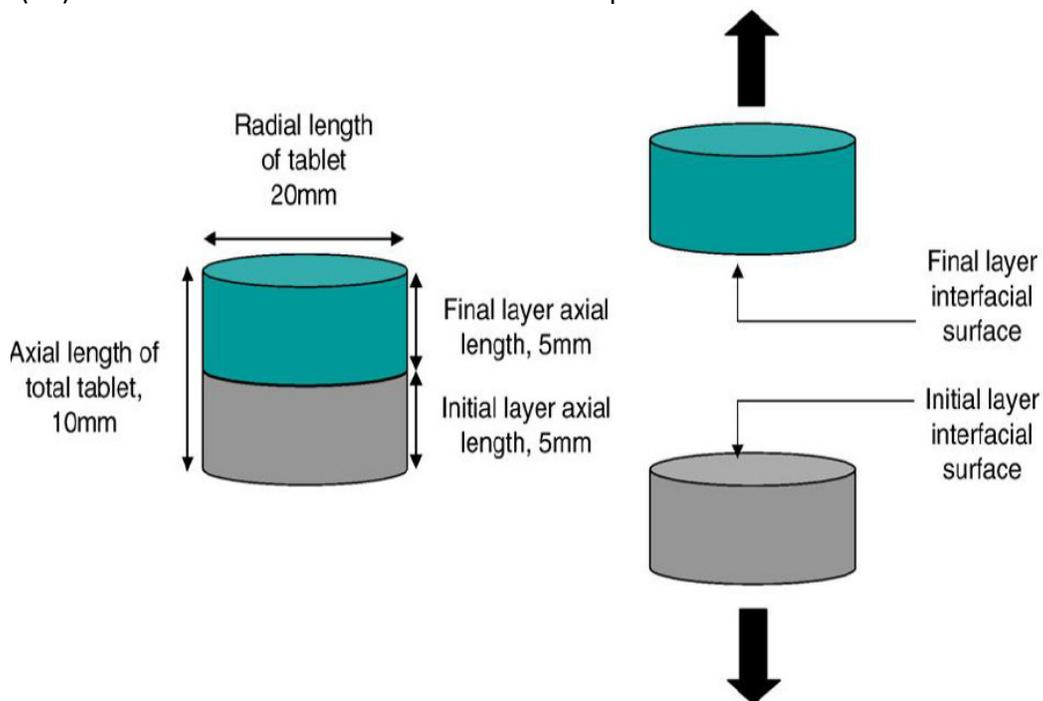
**FIG. 3:** DIAGRAM SHOWING THE DEFINITIONS OF THE AXIAL LENGTHS, RADIAL LENGTH AND INTERFACIAL FRACTURE SURFACES
