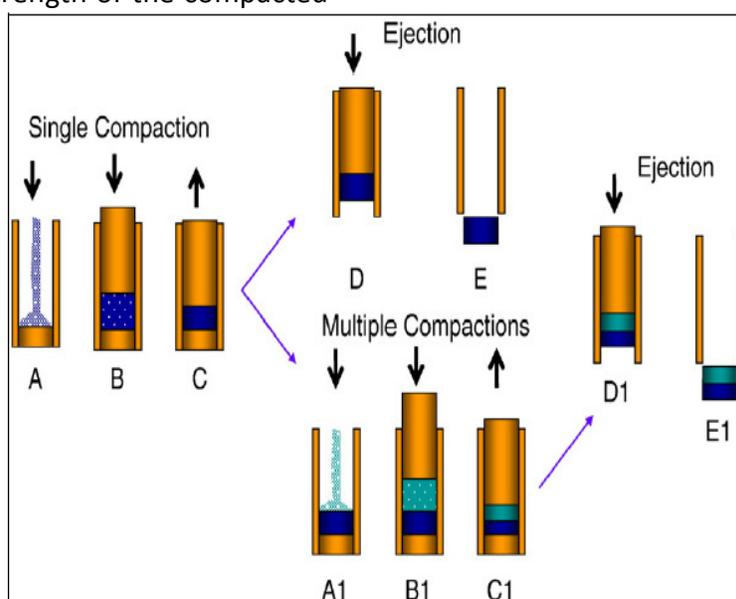
**FIG. 2:** SCHEMATIC DIAGRAM SHOWING THE MANUFACTURE OF SINGLE AND BILAYER TABLETS UTILIZING UNIAXIAL COMPACTION. A- DIE FILLING, B- COMPRESSION, C- DECOMPRESSION, D- LOWER PUNCH REMOVAL AND REAPPLICATION OF LOAD TO THE UPPER PUNCH, E-TABLET FULLY EJECTED. 1 REFERS TO THE FINAL COMPACTION CONDITIONS
