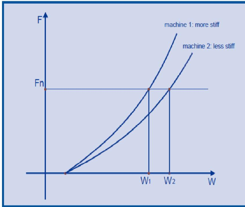
**Graphis 5:** Force and displacement profiles at pre-compression using air Compensation
