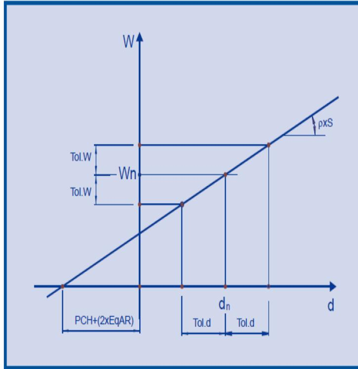
**Graphics 3:** Force tolerance as a function of weight tolerance
