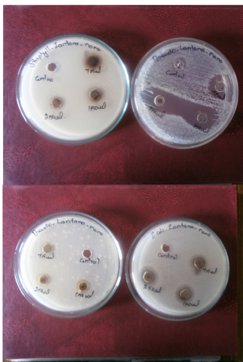
Figure 4. Antimicrobial activity of synthesized silver nanoparticles against S. aureus , E.coli , P. aeruginosa and P. vulgaris
