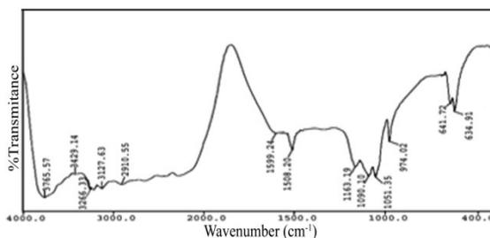
**Fig. 3** FTIR spectra of CuO nanoparticles.
