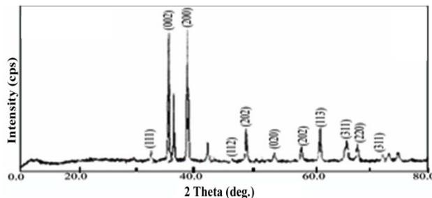
**Fig. 2** XRD patterns of CuO nanoparticles.
